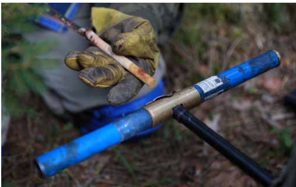
Figure 7.2. Collecting a tree ring sample (increment core) using an increment borer (photo K. Pilch)
